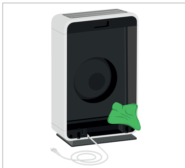
Fig. 17: Cleaning the filter housing
