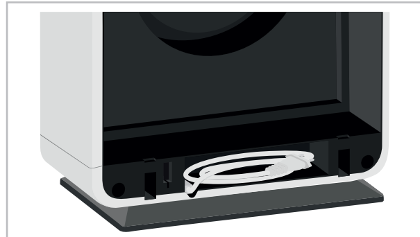
Fig. 11: Transport compartment connection cable
